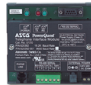
Fig. 17: Telephone Interface Module
