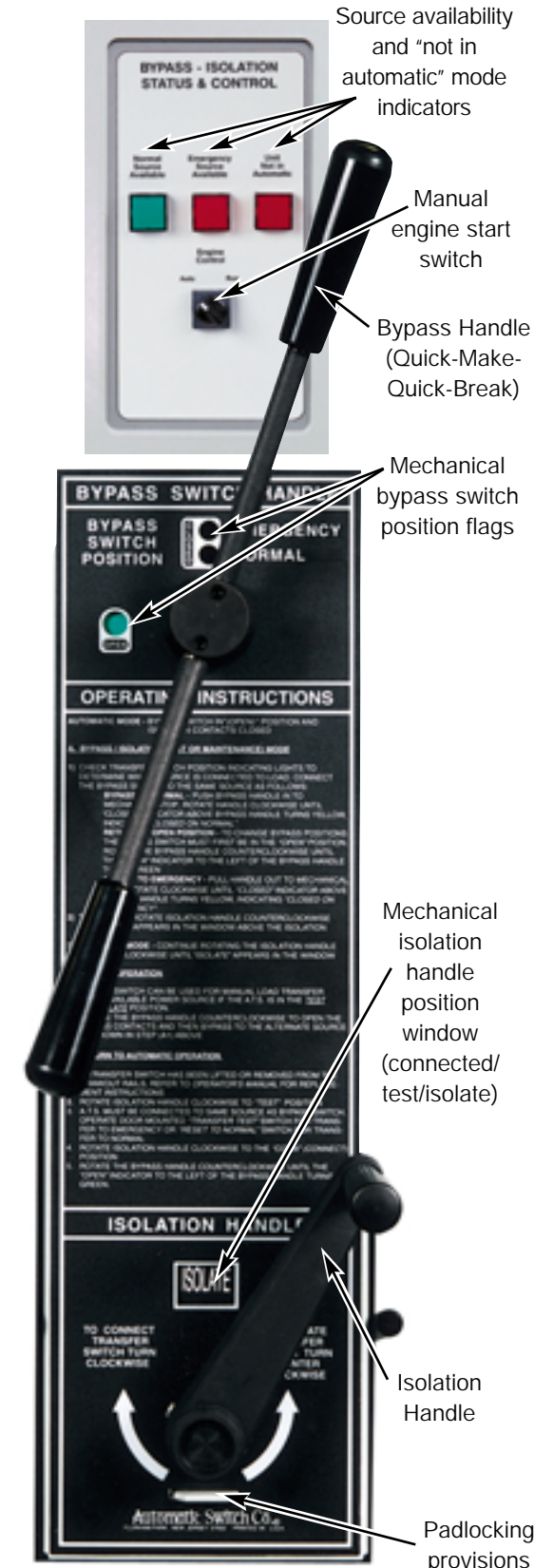
Fig. 8 Bypass-Isolation Switch user interface (1000-3000 amperes shown).
