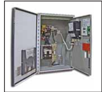
Fig. 17: ASCO Service Entrance Power Transfer Switch rated 2 pole 200 amperes shown in reduced type 3R enclosure where space is limited
