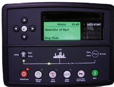
The 7420 controller is an auto start mains (utility) failure module for single gen-set applications. This controller includes a backlit LCD display which continuously displays the status of the engine and generator at all times.
